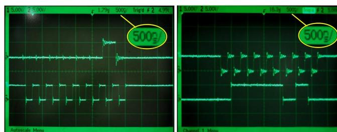
**Figure 15** Results of Master/Slave SPI communications: data *byte* and address *byte*
